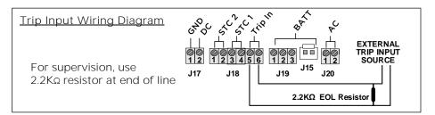
Be sure to use a UL-approved 2200-ohm resistor if the trip input circuit will be supervised (e.g., Bosch P110BL, Bosch EOL-22K, Elk ELR 22). The trip input circuit is not supervised for grounds.
